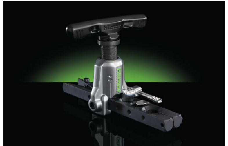
The hilmor Orbital Flare is designed to produce quality flares frequently and conveniently and can be used on mini splits. It’s equipped with a spring-loaded block to firmly grip the tube, a tube-stop arrow for precise height and positioning, and ball detents for easy flaring yoke alignment.
